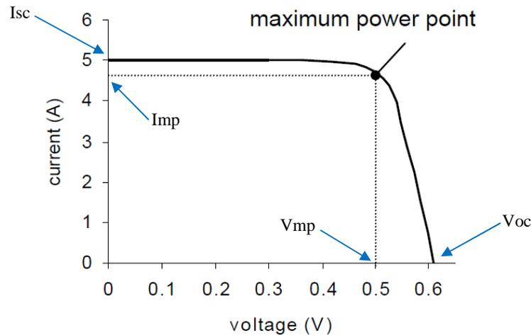
We use the Imp of the solar panels to size the maximum solar charge current for the regulators. Plasmatronics PL and Dingo regulators have a built-in current limit so there is a small margin to play with. 10% extra is no problems for the regulator. For example, the PL20 is designed to limit the current at 20A maximum and even has a temperature sensor onboard that will also reduce the charge current if the regulator gets too hot, so it's very robust.
