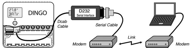
supplies the power to operate it's side of the D232. On the other side, a small amount of power will be drawn from the serial port of the connected device.
