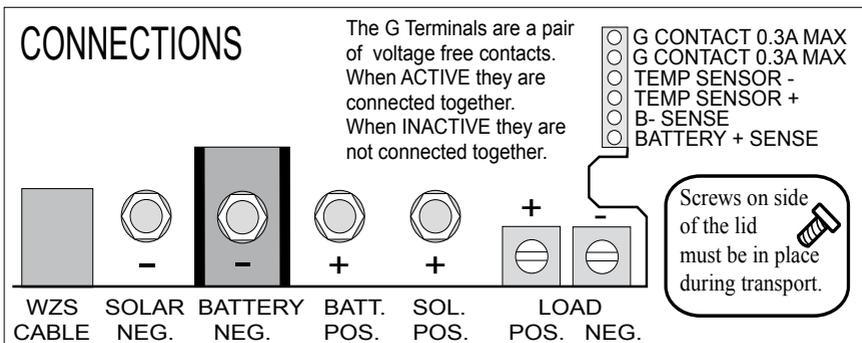
Secure wires to these terminals *tightly*
